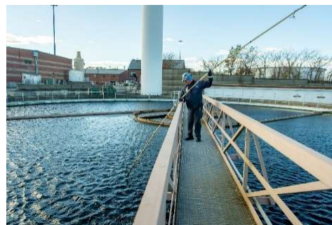
Measuring Depth of Sludge Blanket in Final Clarifier Photo by Peter Goldberg
