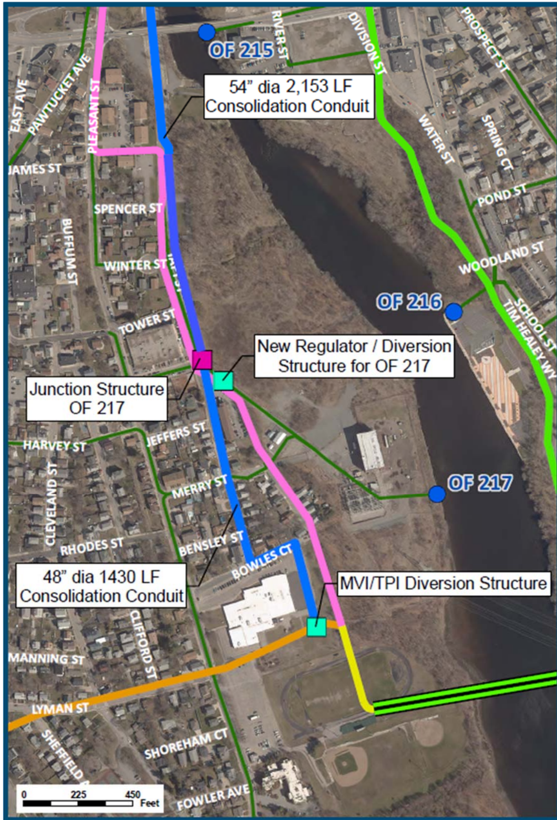
Figure 3.11. Alternative 3 Consolidation Conduit from OF 217
