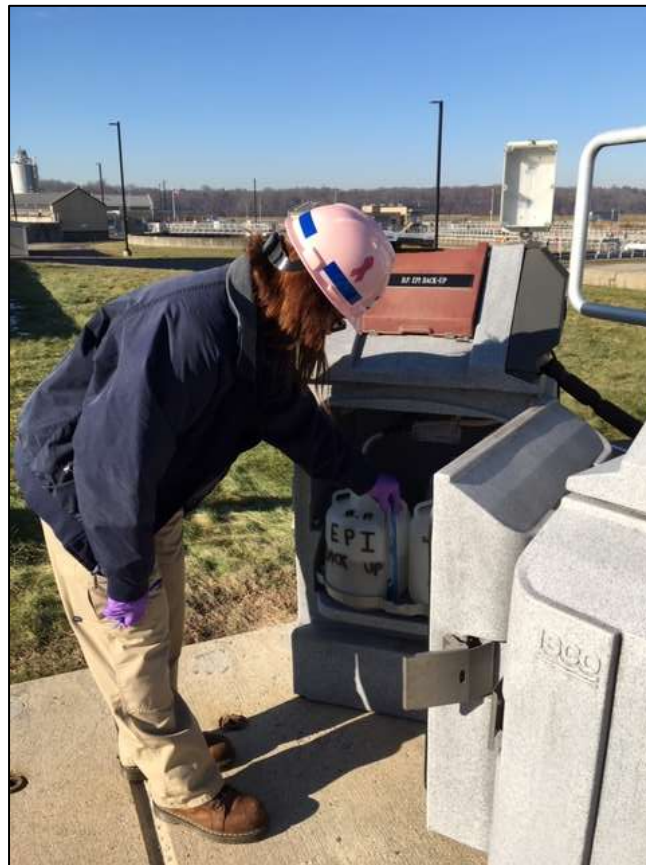
Environmental monitor checking the sampling equipment at the Bucklin Point WWTF.
